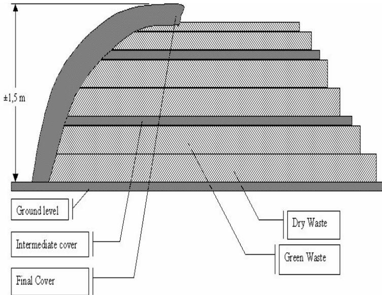
*Figure. 2: Cross section of a windrow compost pile*
